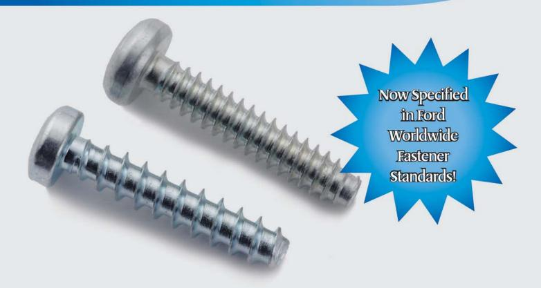
The REMFORM® Screw is a thread rolling fastener with a unique thread form to provide superior performance in today's wide range of plastics. The asymmetrical thread minimizes radial hoop stress to reduce boss bursting. The narrow tip angle also reduces stress in the plastic nut member.
