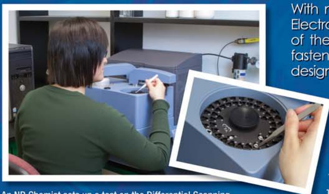
An ND Chemist sets up a test on the Differential Scanning Calorimetry machine.
