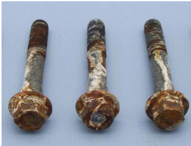
FIGURE 1: PART EXAMPLES AFTER SALT SPRAY TESTING
