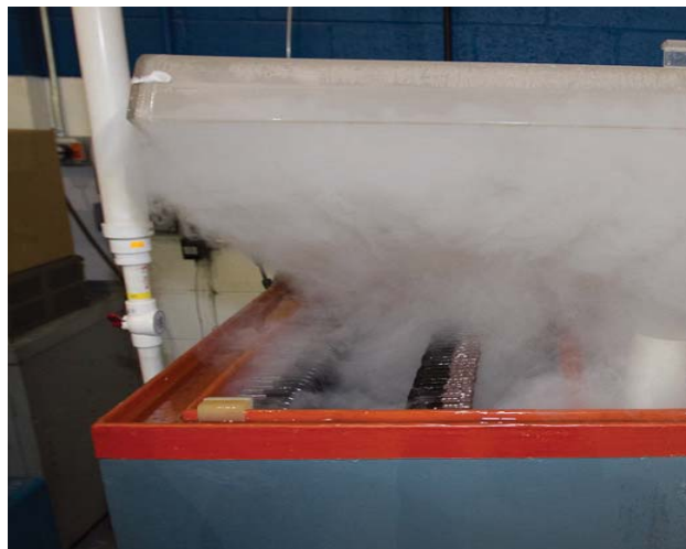
FIGURE 2: TYPICAL VIEW INSIDE A SALT SPRAY CHAMBER
