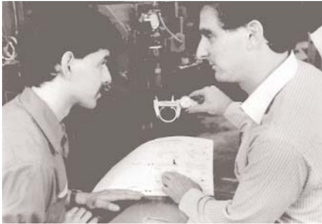
QUALITY INNOVATIONS IN THE 1980's INCLUDED "IN PROCESS" CHECKING. ROTOR CLIP QA MANAGER BRUCE RUDIN INSTRUCTS A PRESS OPERATOR HOW TO MEASURE THE FREE DIAMETER OF A RETAINING RING WITH A VERNIER INTERFACED TO A COMPUTER. (PHOTO CIRCA 1985. NOTE BRUCE RUDIN IS STILL WITH ROTOR CLIP!)
