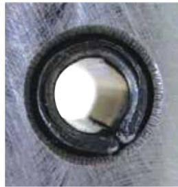
at the same location. The thinner material on the ISO 13337 light duty Slotted Pin is not able to easily absorb this additional material stress, and premature fatigue results in assembly failure.
