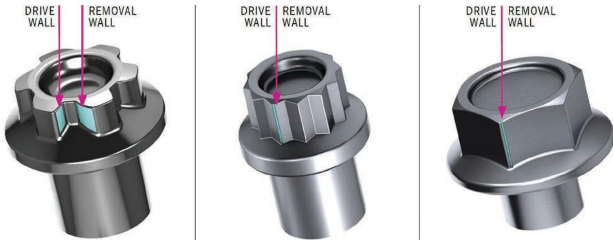
**THE ASYMMETRIC LOBES OF THE EXTERNAL MORTORQ® SUPER BOLT HEAD PROVIDE LARGE CONTACT SURFACES WITHOUT THE TALL HEAD HEIGHT REQUIRED FOR HEX AND 12 POINT HEAD BOLTS.**
