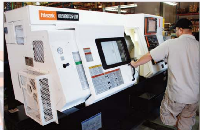
Mazak Nexus Quick Turn CNC Lathe – 3" Thru the Spindle Capacity, and 14.75 Diameter X 19.85 Length Chucking Capacity
