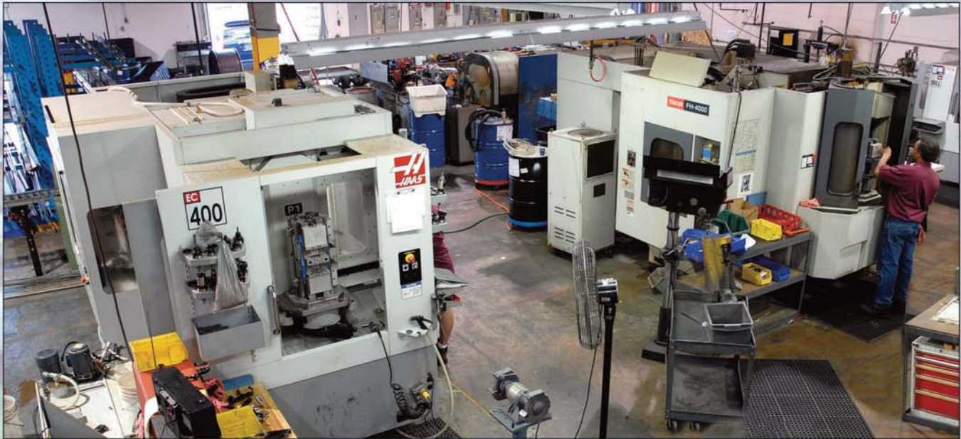
Milling Centers – (2) Horizontal Double Pallet 400MM CNC Milling Machines from Mazak and Haas
