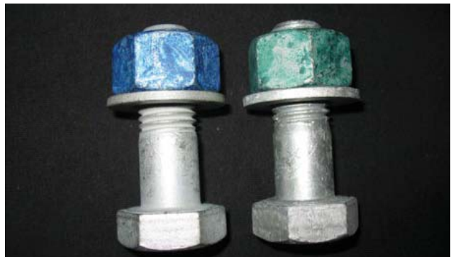
Figure 2: Mechanically galvanized fasteners (left, blue nut) have a dull flat gray finish compared to the shiny appearance of hot-dipped galvanized fasteners (right, green nut).
