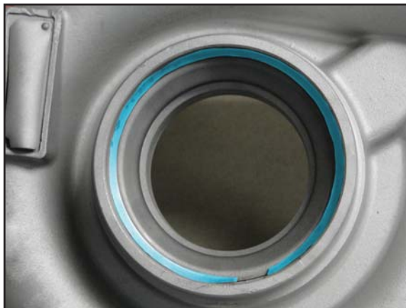
A "Silencer Ring" (above) prevents the whistling sound associated with turbochargers. It is held in place by a Rotor Clip constant section retaining ring (below).
