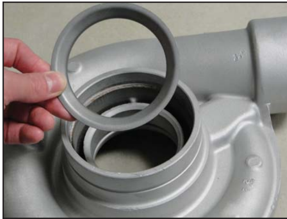
A "Silencer Ring" (above) prevents the whistling sound associated with turbochargers. It is held in place by a Rotor Clip constant section retaining ring (below).
