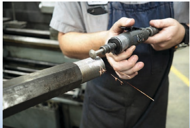
MODEL 752 AND A MANUFACTURER USING TOOL TO DO MINOR PRODUCTION TOUCH-UPS ON MISS-HANDLED INVENTORY.
