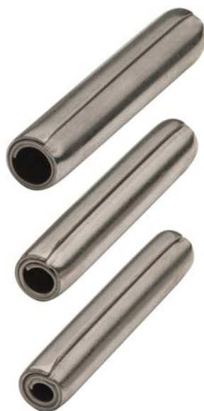
SPIROL COILED SPRING PINS ARE AVAILABLE IN THREE "DUTIES" (PICTURED FROM TOP: LIGHT, STANDARD, HEAVY) TO ENABLE THE DESIGNER TO CHOOSE THE OPTIMUM COMBINATION OF STRENGTH, FLEXIBILITY AND DIAMETER TO SUIT DIFFERENT HOST MATERIALS AND APPLICATION REQUIREMENTS.
