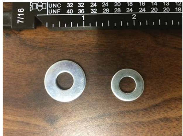
5/16 DIAMETER USS AND SAE FLAT WASHERS. WHICH IS LARGER? THE USS WASHER WILL ACTUALLY FIT ON A 3/8 BOLT.
