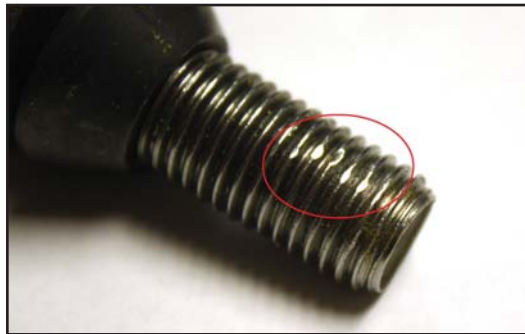
ABOVE: DEFECT FOUND ON PART WITH LASERLAB
