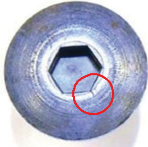
FIGURE 3: FORGING CRACK AT EDGE OF RECESS
