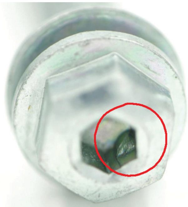
FIGURE 9: PARTIALLY BROKEN PUNCH
