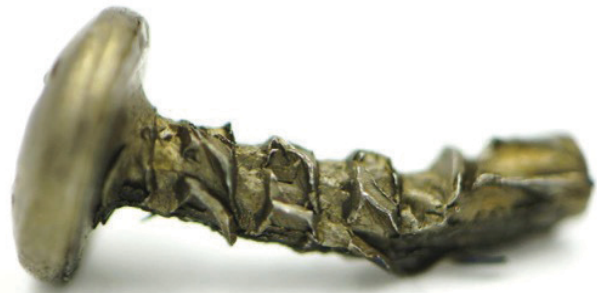
FIGURE 11: PART THAT SLID THROUGH ROLL DIE
