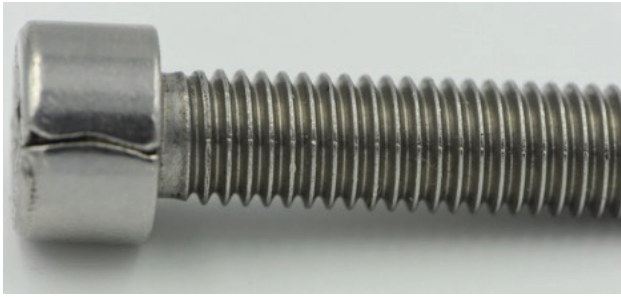
FIGURE 1: CRACK FROM WIRE SEAM
