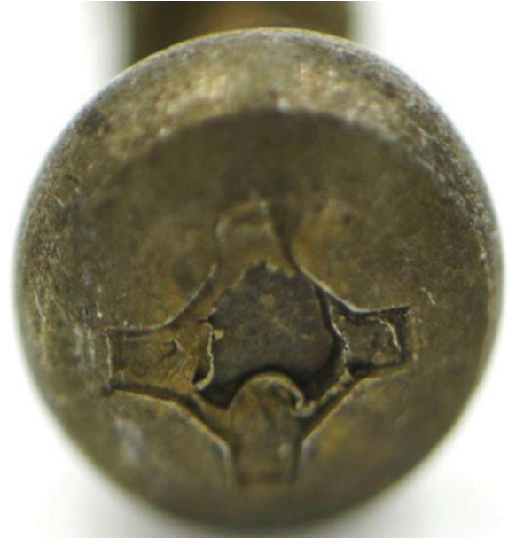
FIGURE 8: FULLY BROKEN PUNCH
