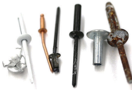
IMPROPER REPROCESSING CAN CAUSE RIVET FAILURE IN MANY WAYS INCLUDING CRACKING PAINT, BENT MANDRELS AND RUST.
