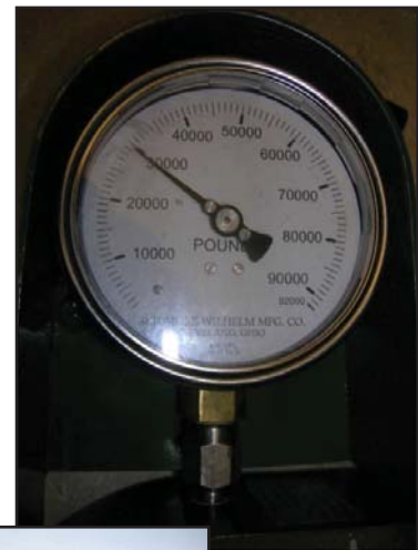
Figure 2: Galvanized A325 Bolt; Tension at 1/3 Turn 30 kips vs. 41 Minimum
