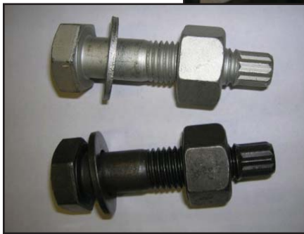
Figure 1: Plain and Coated TC Bolts; Coated TC Bolt Tension 26 kips vs. 41 kips Minimum
