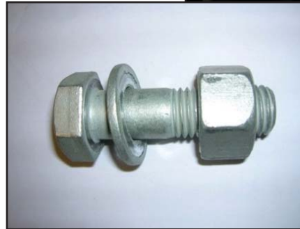
Figure 2: Galvanized A325 Bolt; Tension at 1/3 Turn 30 kips vs. 41 Minimum
