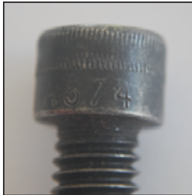
ABOVE: ASTM A574, knurl pattern identifies manufacturer
