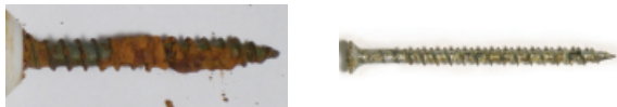
(Left to right): polymer coated fastener after exposure to wood extracts, electroplated fastener after exposure in solid wood.
