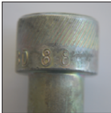
BELOW: Side marking of an 8.8 metric SHCS
