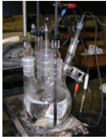
Electrochemical test cell.
