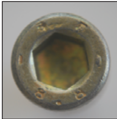
ABOVE: Marking on top of socket head indicating an 8.8 metric
