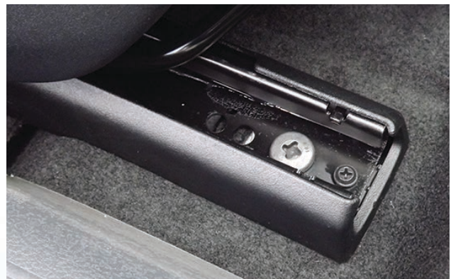
MORTORQ SUPER FASTENERS HOLD THE SEATS IN PLACE FOR FCA.
