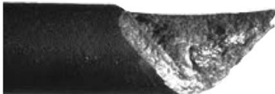
FIGURE 6: PURE TORSION FAILURE
