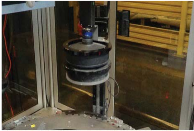
Figure 3: Vertically mounted camera for head cracks
