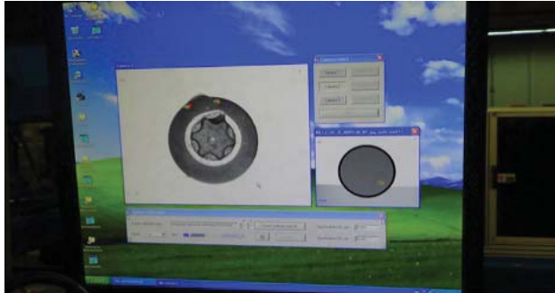
Figure 8: Sample Screen Shot of Cracked Head Detection
