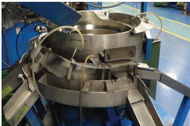
Figure 2: Bowl Sorter (Note chutes for suspect material on left)
