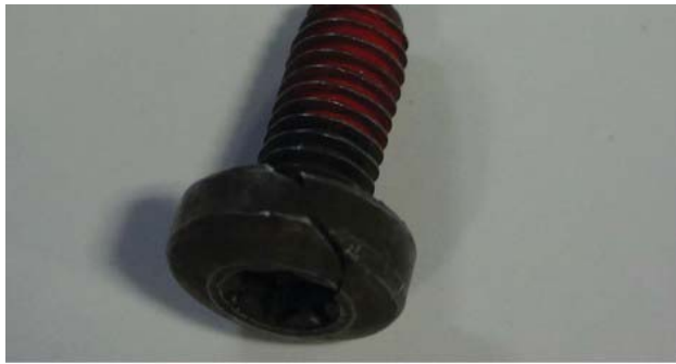
Figure 7: Typical Compression Cracked Head
