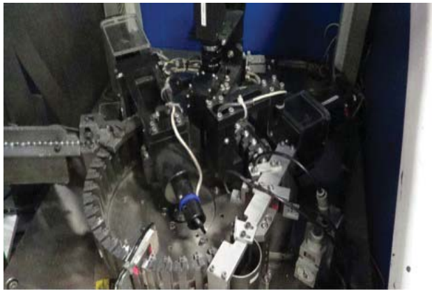
Figure 4: Multiple Camera Sorter- Mounted horizontally and vertically
