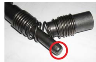
Figure 3: Worn insertion quill.
