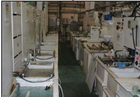
CSL Inc. has developed a cad-free plating process that delivers electrical conduction and corrosion resistance and is RoHS compliant. EN-PTFE cross mates with stainless steel, aluminum PEI, and PEEK and other metals and composites.
