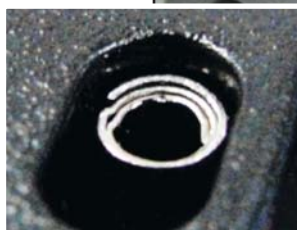
Figure 4: Using an improper installation tool will make the pin telescope or unwrap.
