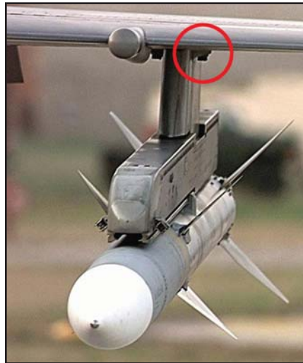
Spiralock 1/4-28 tapped holes are used for mounting connections under aircraft wing on this F-18 Hornet/A1N-120 AMRAAM Air-to-Air Missile
