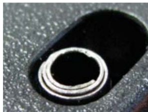
Figure 5: Flip side of the same installed pin.
