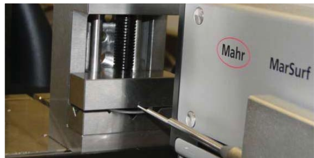
Above: A dual stylus ensures accuracy by measuring the top and bottom of the ring without having to re-position it as required if using a single stylus.
