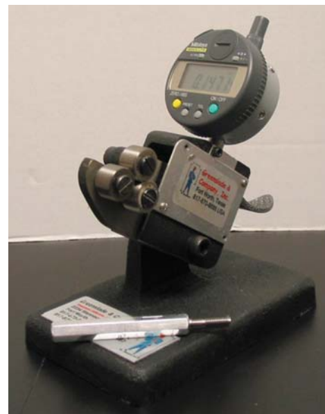
TYPICAL EXTERNAL VARIABLE THREAD GAGE – "TRI-ROLL" GAGE
