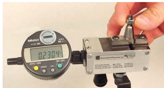
TYPICAL INTERNAL VARIABLE THREAD GAGE - "BI-POINT GAGE"
